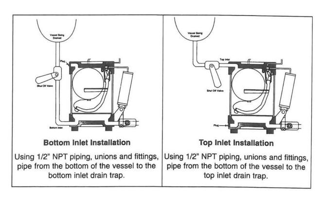
Completed piping should enable the condensate to flow continuously downward into the trap.
