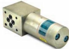
Adjustment of the outlet pressure is carried out by varying the supplied pressure,  $P_H = (P_{IN} - P_{Return}) i$ , where  $i$  equals intensification.
